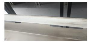
(3) Steam tubes are made of SS316 with rubber wrapping.
